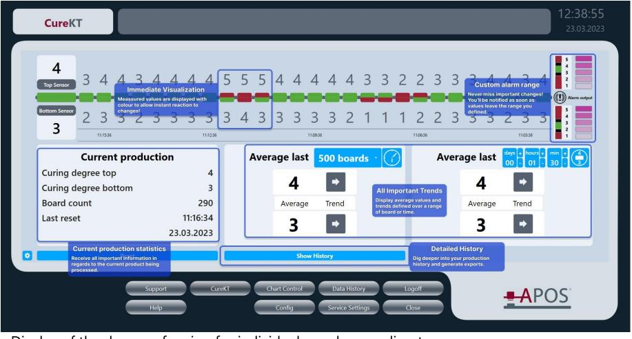
Display of the degree of curing for individual panels according to production sequence
