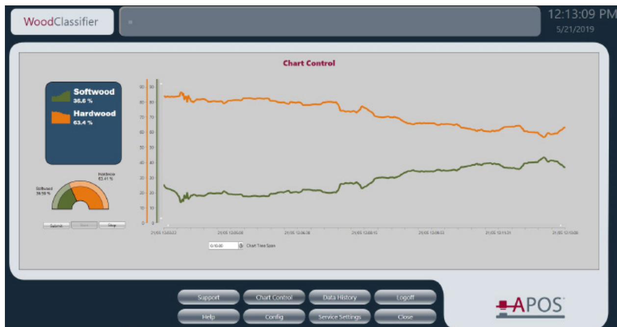
Figure: Screenshot WoodClassifier (single sensor system, double sensor possible)
